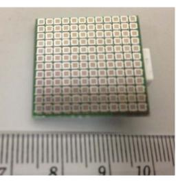
SiPM 1.6 x 1.6 mm<sup>2</sup> of 1.9 mm pitch based on PM1150 (KETEK)
